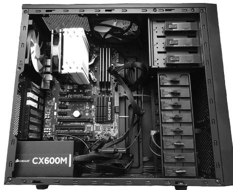
Figure 1: The inside of a desktop PC
