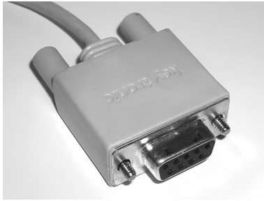
Figure 11-15: A traditional serial port connector
