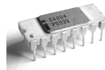
Figure 1-29: An Intel 4004 chip in its packaging
