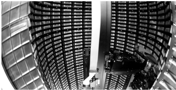
Figure 10-21: A robotic tape jukebox in a data center
