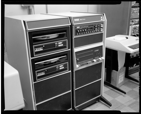
Figure 1-27: A transistor-based 1960s PDP-11 mini-computer
