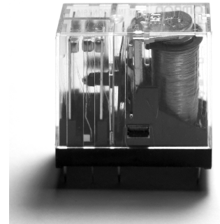
Figure 1-17: A relay showing a wire coil
