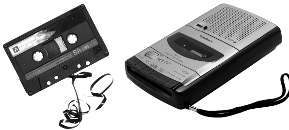
Figure 10-13: A 1980s compact cassette and player/recorder, used for both analog music and digital file storage
