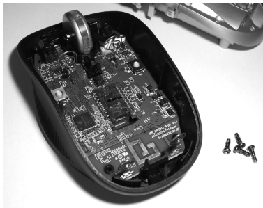
Figure 13-10: The inside of an optical mouse
