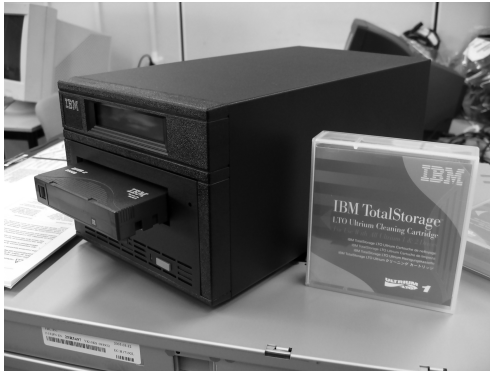
Figure 10-14: An IBM Ultrium Linear Tape Open cartridge and drive
