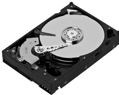
Figure 10-19: The inside of a magnetic hard drive
