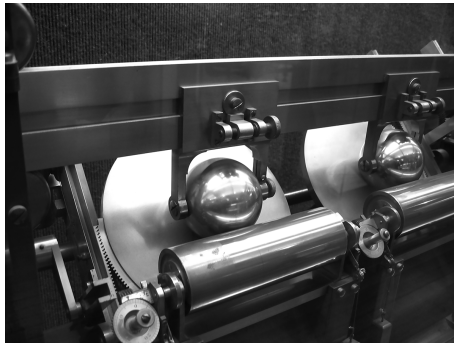
Figure 1-16: A ball and disc integrator from Kelvin's differential analyzer
