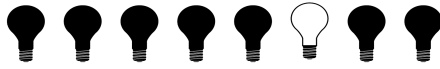
Figure 2-9: A representation of the number 5 in a one-of- N system (the leftmost bulb represents 0)
