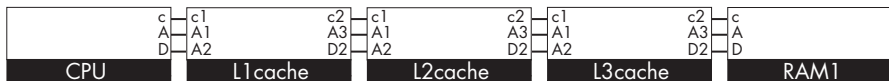
Figure 10-9: A basic CPU, bus, and RAM architecture with L1, L2, and L3 caches
