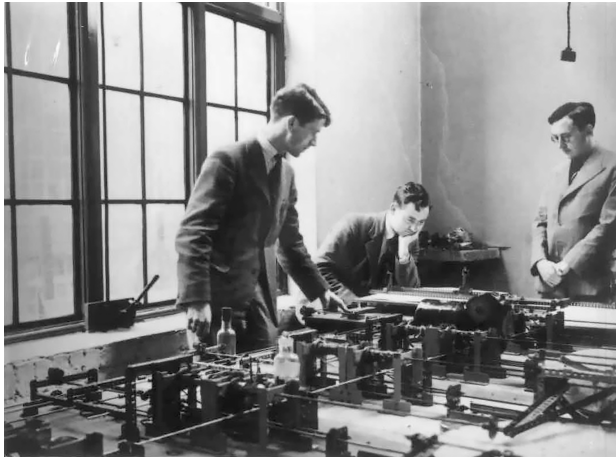
Figure 1-19: Maurice Wilkes (right) with the mechanical Cambridge Differential Analyzer, 1937
