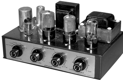
Figure 1-21: A guitar amplifier made with vacuum tubes
