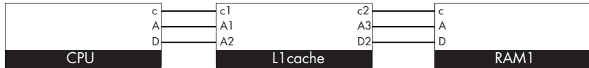
Figure 10-8: A basic CPU, bus, and RAM architecture with a cache in between
