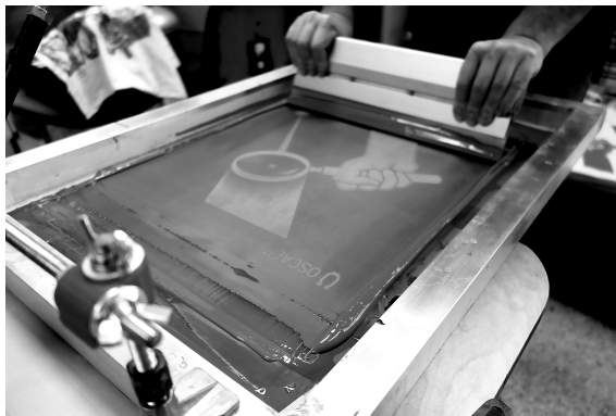
Figure 3: To print this poster, a silk screen mask is placed on a piece of paper, and paint is pushed through it using a squeegee.
