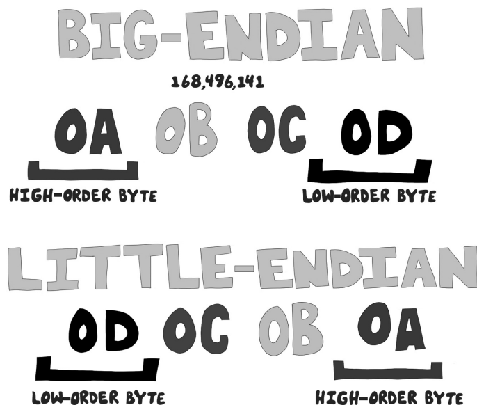
Figure 4-16: Big-endian versus little-endian byte order
