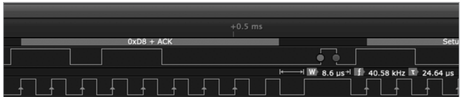
Figure 8-4: A stretched clock signal reduces the triangle wave frequency.
