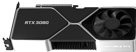
Figure 13-6: A 2022 Nvidia RTX 3080 GPU
