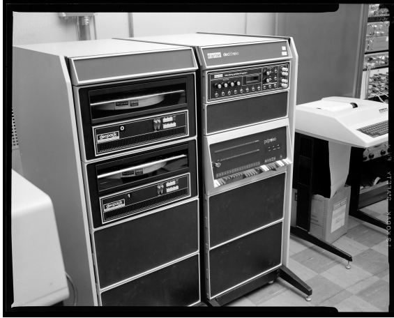
Figure 1-27: A transistor-based 1960s PDP-11 mini-computer
