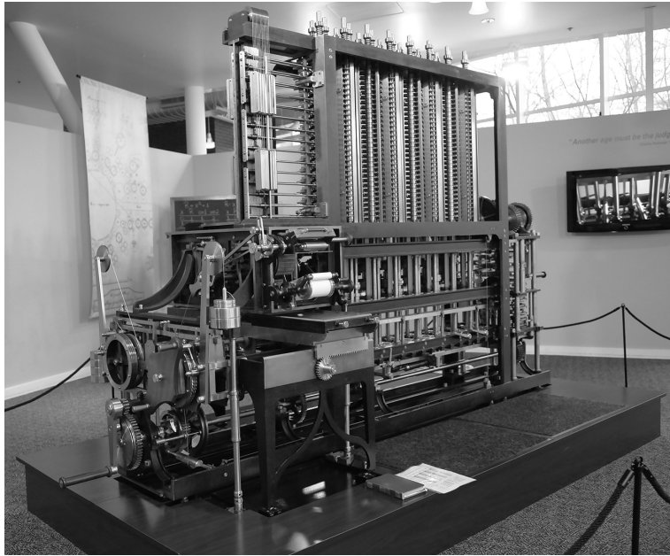
Figure 1-13: A metal rebuild of Babbage's Difference Engine
