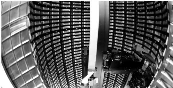
Figure 10-21: A robotic tape jukebox in a data center
