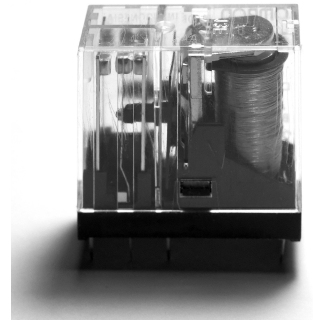
Figure 1-17: A relay showing a wire coil
