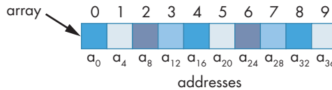
Figure 9-7: The layout of a ten-integer array in memory. Each a_i -labeled box represents an offset of four bytes, as each integer requires four bytes to store.
