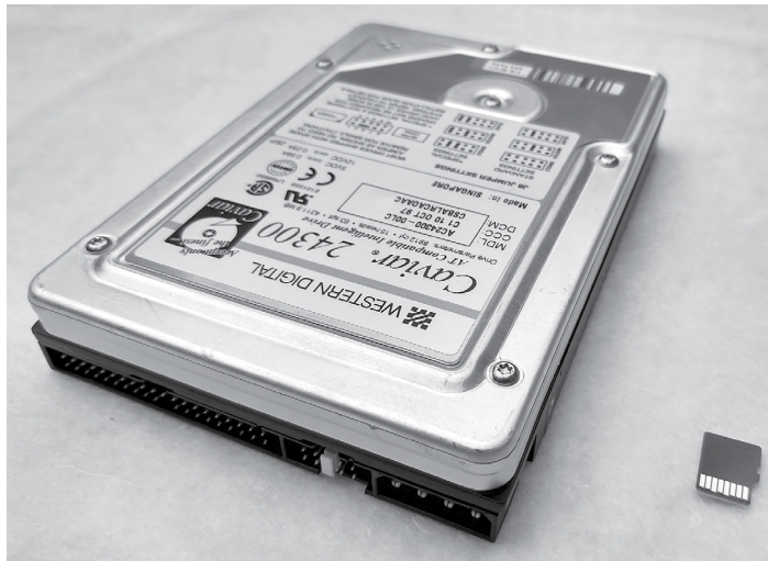
Figure 7-12: A 4GB hard disk drive from 1997 beside a modern 32GB microSD card, a type of solid-state storage
