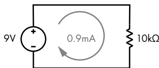
Figure 3-5: The flow of current illustrated as a loop
