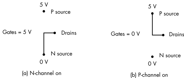
Figure 5-15: CMOS inverter equivalent circuit: (a) pull-up open and pull-down closed, (b) pull-up closed and pull-down open
