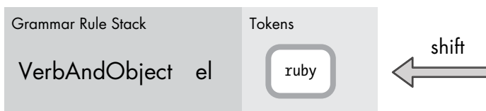
Figure 1-23: The parser shifts another token onto the stack.
